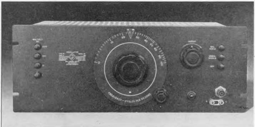
Figure 1. Panel view of the Type 1302-A Oscillator.
